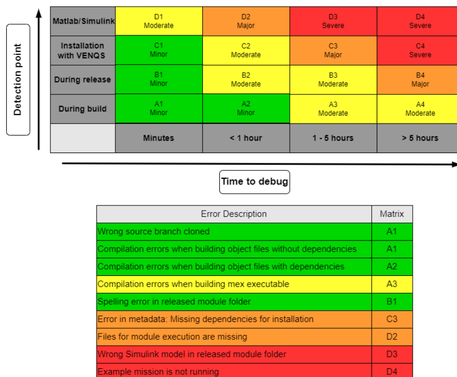
Figure 2: Overview of errors for module releases faced before CI/CD implementation based on a 4x4 risk matrix schema
