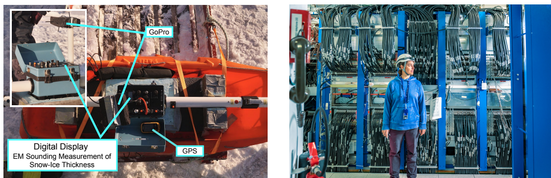
Figure 1: (Left) A rudimentary form of instrument orchestration: A GoPro camera is depicted here being used to record data from the digital display of a Geonics EM31-ICE for snow-ice thickness measurements. The footage is matched to GPS data to build a location-resolved data series [NP24]. Illustration adapted from [Fou24b]. (Right) In comparison, an advanced experimental control system at CERN/ATLAS, the Trigger and Data Acquisition system, which is used to pick out distinguishing events and reduce data flow [CER25]. Photo from [CG20].
